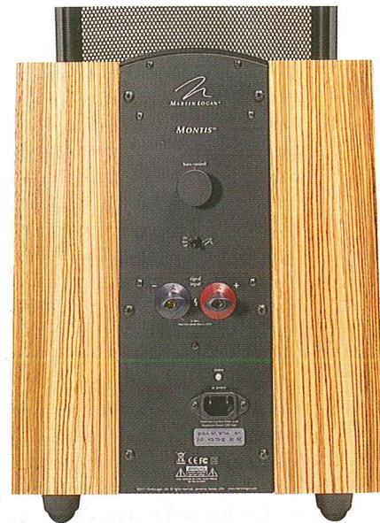
The rear panel carries a single pair of inputs: bi-wiring is not possible. They accept 4mm plugs, spades and bare wires. A bass level control and light switch sit above.
